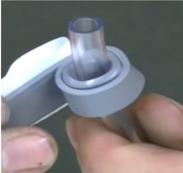
Figure 7. Gum tape applied to vacuum tubing.
